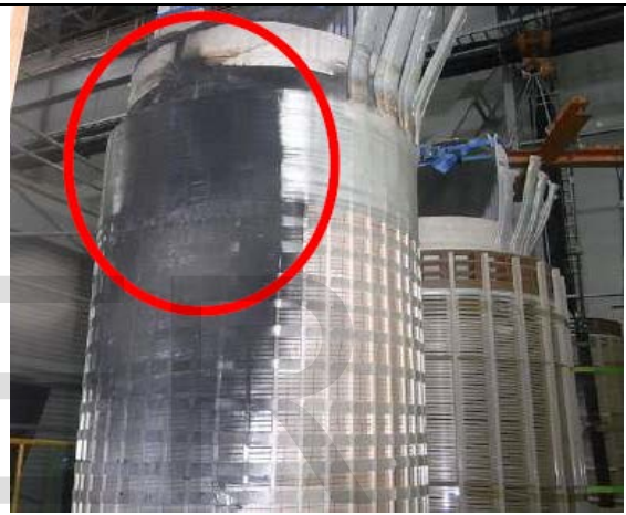
Fig 3. The short circuit fault was copper wire-exposed yielded because the insulation paper deteriorated between winding the insulation layer.
